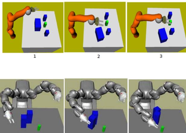
Figure 2: Motion planning for grasping allowing the interaction with obstacles.
